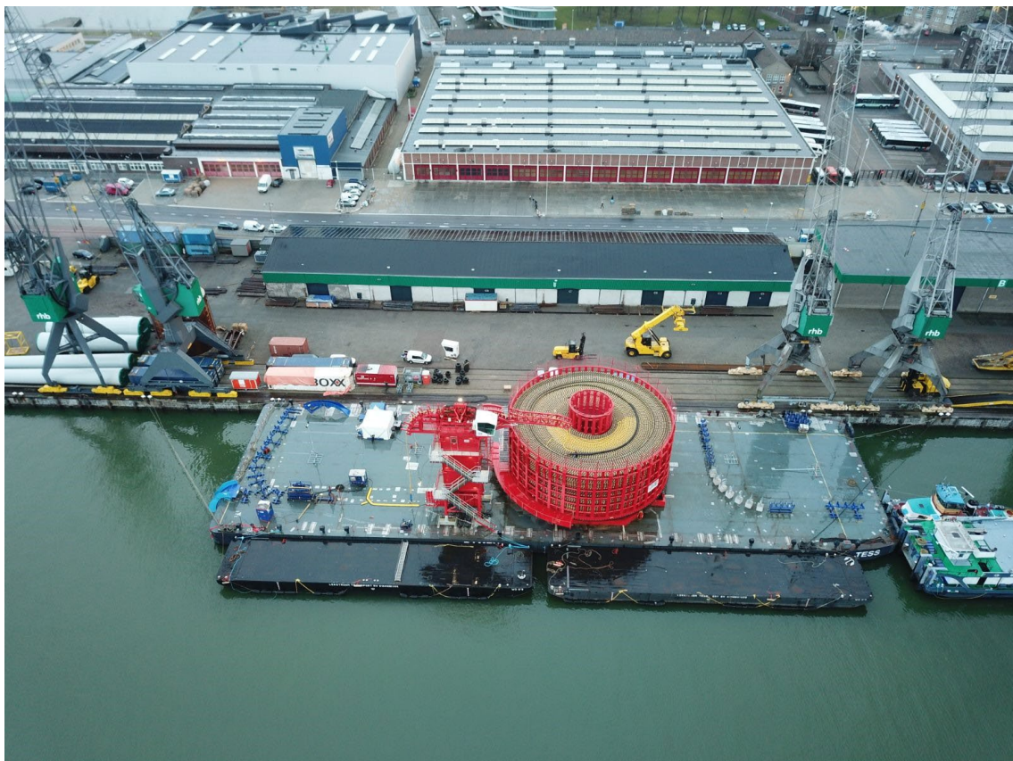
Figure 1 • Blue Offshore's BC01 23m OD, 10m fill height, mobilized on DAMEN TESS in Rotterdam, NL.
