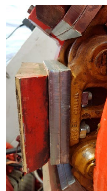
Figure 2 • Modified trackpads to handle project diameters
