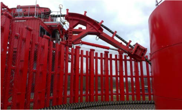
Figure 2 • Loading arm from within basket carousel.
