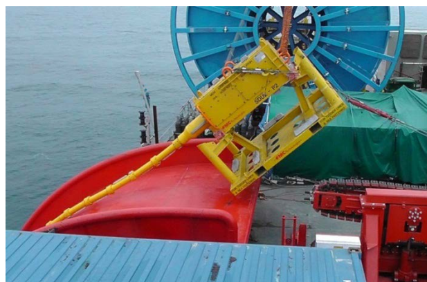
Figure 6 • SDU 1 in position on chute.
